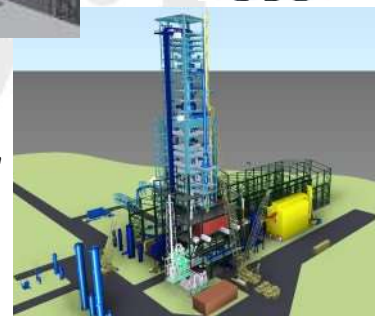
Integrated Process Scheme for Production of Hot Metal with Natural Gas: ENERGIRON ZR + Tenova OSBF
